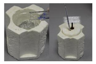
**Purpose:** To calculate enthalpy change of a reaction by using calorimeter and understand the difference between endothermic and exothermic reactions
