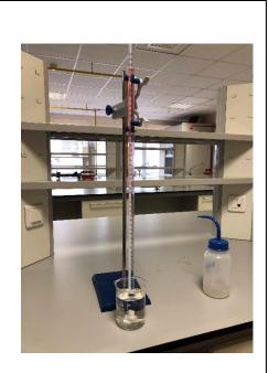
8. Make sure the cotton is stacked at the end of burette. When the system is shown to be airtight, wait until the acid solution comes in contact with the metal. You will see the hydrogen gas is being produced as bubbles near the metal, and some water will pour into the beaker.
