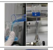
**3.** Slowly add hot  $CuSO_4$  solution to the beaker that contains the iron powder. Stir the mixture a few times until completeness of the reaction. You should see copper forming. When the reaction has finished, allow the copper product to cool.
