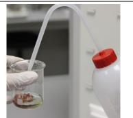
6. The acetone readily dissolves the water and helps the removal of it from the medium. Swirl the beaker gently on low heat flame. Copper product should be spread in a single layer on the bottom of the beaker. Grinding of aggregates with a spatula makes the copper easy to dry. Be sure not to remove any copper from the beaker.
