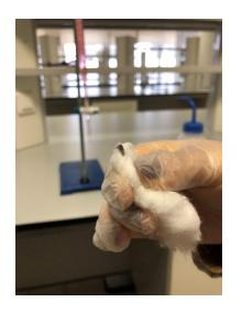
5. Tie this metal in cotton with a piece of thread and hang it a few centimeters above from the top of the liquid in the burette, providing that it does not come into contact with the acid solution. You may drop it into the solution as well.
