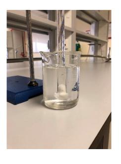
9. After the metal has completely dissolved, read the volume of the water in the burette and record it (V<sub>2</sub>). The displaced amount of water in mL will be taken as the amount of hydrogen gas liberated. Record the room temperature. Record the atmospheric pressure, P<sub>atm</sub> and the vapor pressure of water, P<sub>H<sub>2</sub>O</sup> at this temperature.</sub>
