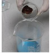
**5.** Add about 10 mL of distilled water to the solid copper and swirl to wash any remaining ions from the copper. Decant the wash water from the copper and add 10 more mL of distilled water, swirl and decant again. Wash copper particles finally with several mL of acetone (**CAUTION**-Acetone is very flammable). Swirl and allow to stand a few minutes. Decant off the acetone.
